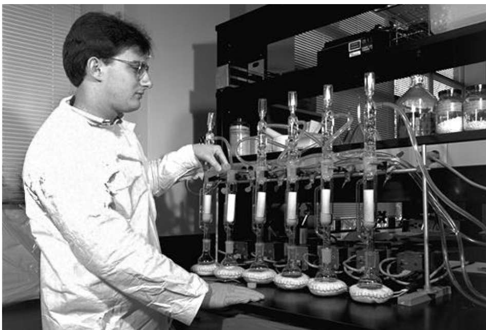
Graduate student Mark Prytula conducts Soxhlet extraction in the lab to help quantify contamination levels in sediment samples from the Bayou d'Inde.
