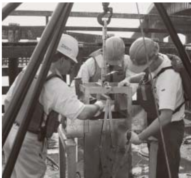
A box corer sample of Anacostia River sediments is prepared for laboratory treatability testing in a demonstration of active capping technologies.
